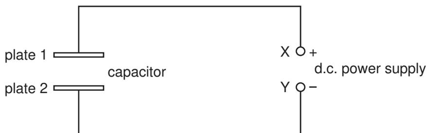
Along which paths do electrons flow as the capacitor starts to charge?
