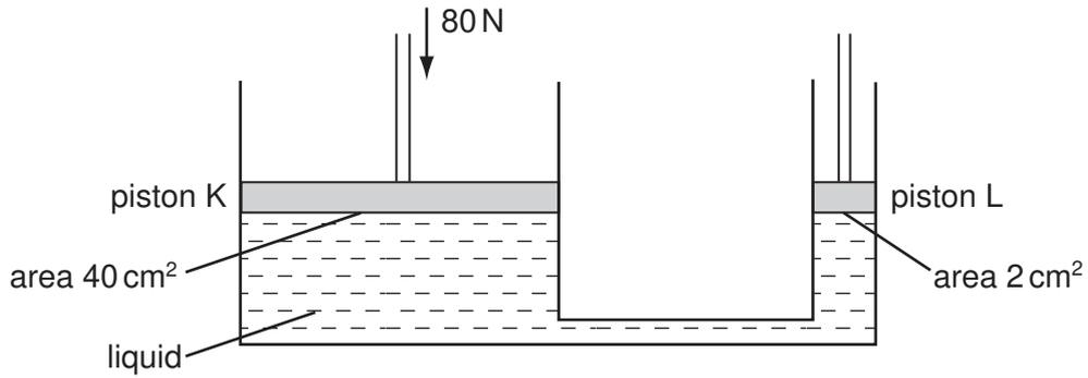
A downward force of 80 N is exerted on piston K.
